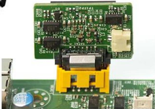
Direct connection to Yellow SATA connector
